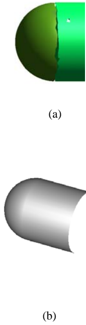
Figure 7: After reduction (a) the data set has been segmented (b) are two faces reconstructed.
